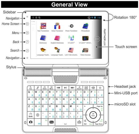
Due to the rotary screen, the device can be easily transformed into a handy tablet. Just turn the device screen 180° clockwise from its original position. To restore the screen to its original position, turn it 180° counterclockwise.
